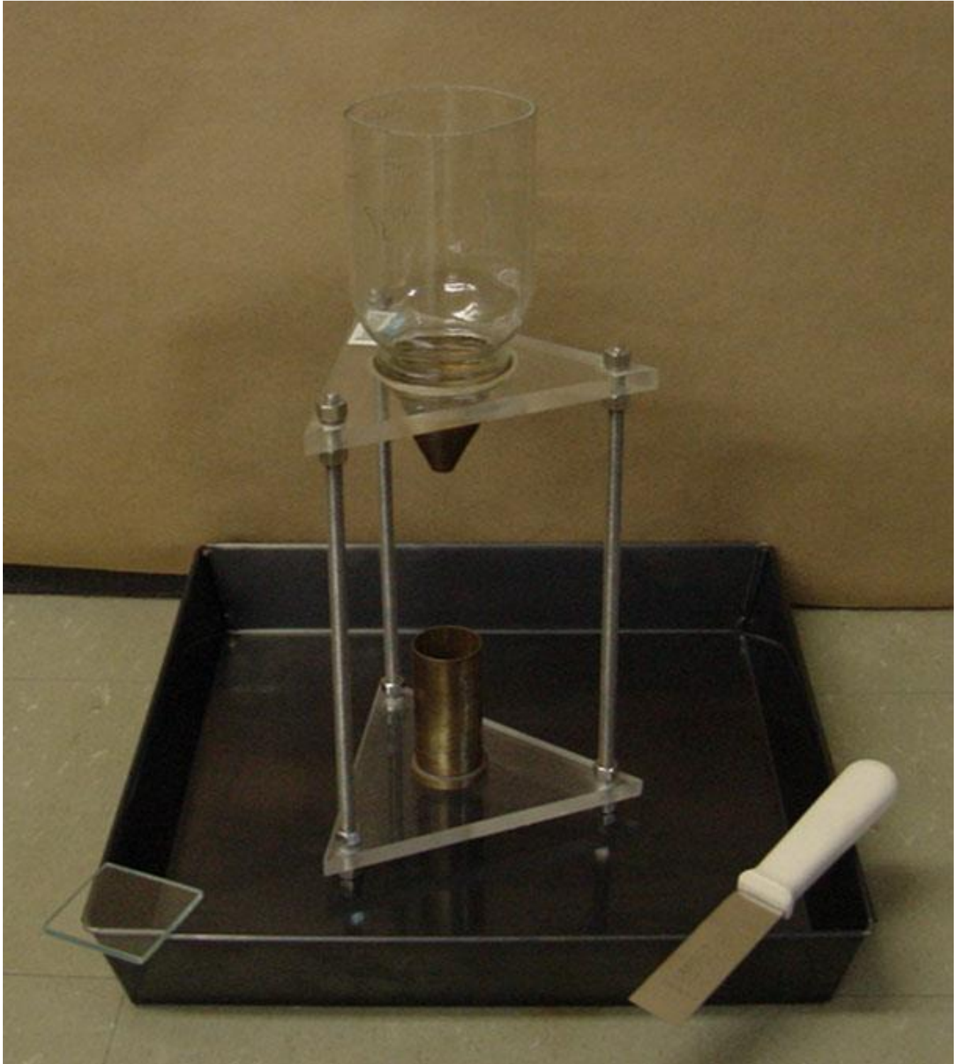
Figure 1 Apparatus (Funnel, Funnel Stand, Cylindrical Measure, Catch Pan, Glass Plate, and Metal Spatula)
