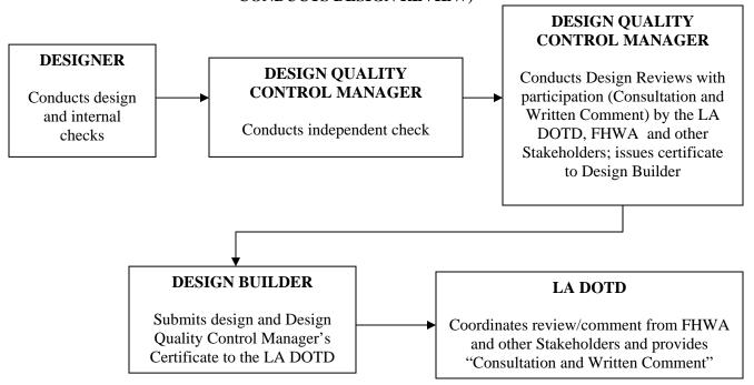
The Design-Builder and the LA DOTD will follow the process shown in Figure 111-12B for As-Built Plan Design Reviews.
