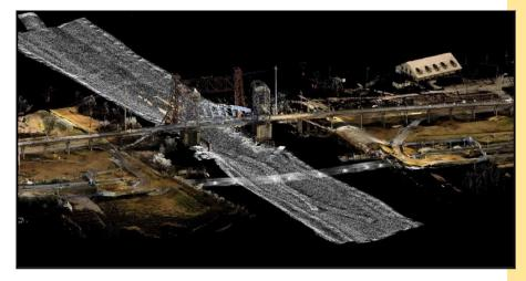
Laser Scan and Hydrographic Survey of Belle Chasse Bridge and Tunnel project area
