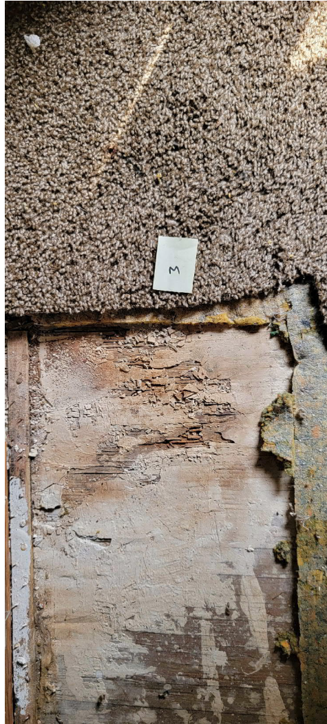
Photograph No. 3 HA-03: Brown Carpet with Yellow Padding and Yellow Leveling Compound
